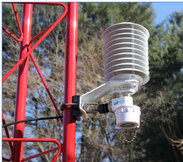
Typical radiation shield installation shown with a Richards high accuracy Platinum RTD temperature sensor and PPSH Weatherproof Junction Box for convenient sensor wiring.
